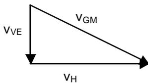
$$V_H = \sqrt{V_{GM}^2 - V_{VE}^2}$$
